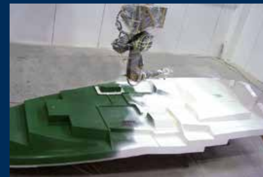
Robot applying gelcoat in the mould
